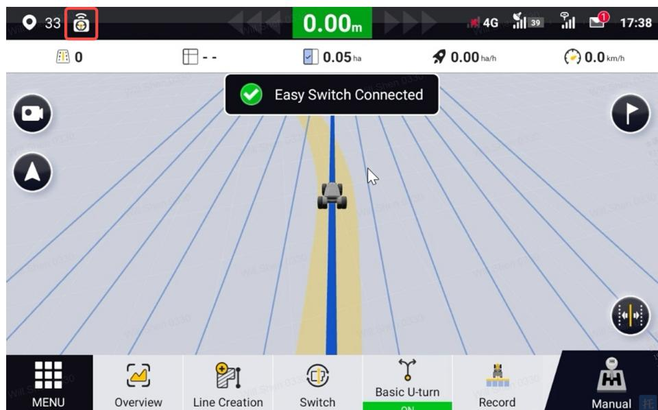
5. Press the hardware button or press the foot pedal to control the automatic/manual driving buttons on the interface.
