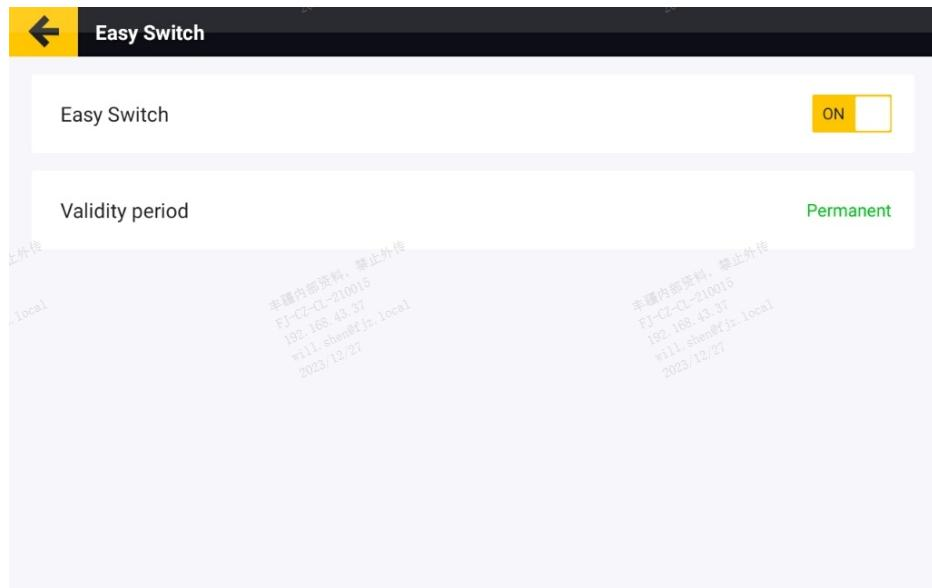
4. Returning to the homepage, when the Easy Switch button is connected and the function is enabled, the button icon will be displayed in the upper left corner.
