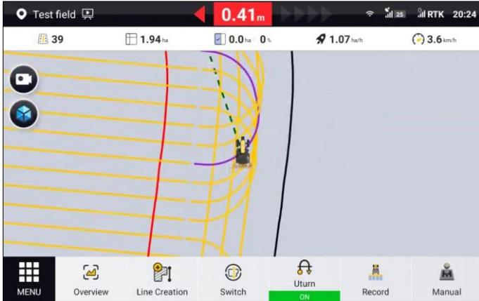
**Figure 111.** Follow the guiding line to the start point
