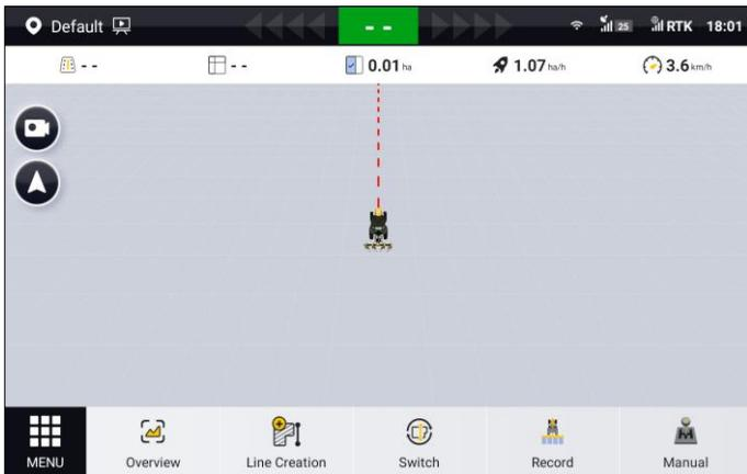
**Figure 73.** Guiding line for resuming a task operation
